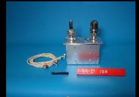
Above: Ion gauge (IOG) system is composed of two sensors with cylindrical and spherical chambers. Left: IOG is mounted at the top stage of mission bay of the S-520-32 sounding rocket
